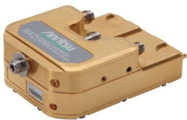
Figure 5: an NLTL-based frequency extension module operating at up to 145 GHz. Weighing just 365g, it is 1/50th the volume of traditional millimetre-wave modules.
